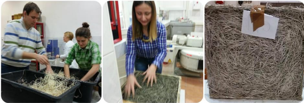
Figure 196 - Our efforts to produce wood wool insulation by ourselves
