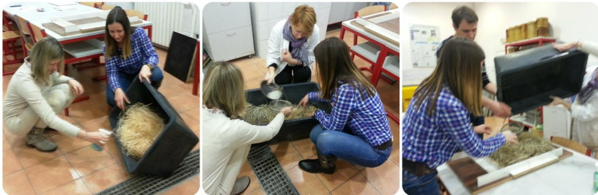
Figure 174 - Spraying wood fibres with water and distributing cement over the wood fibres
