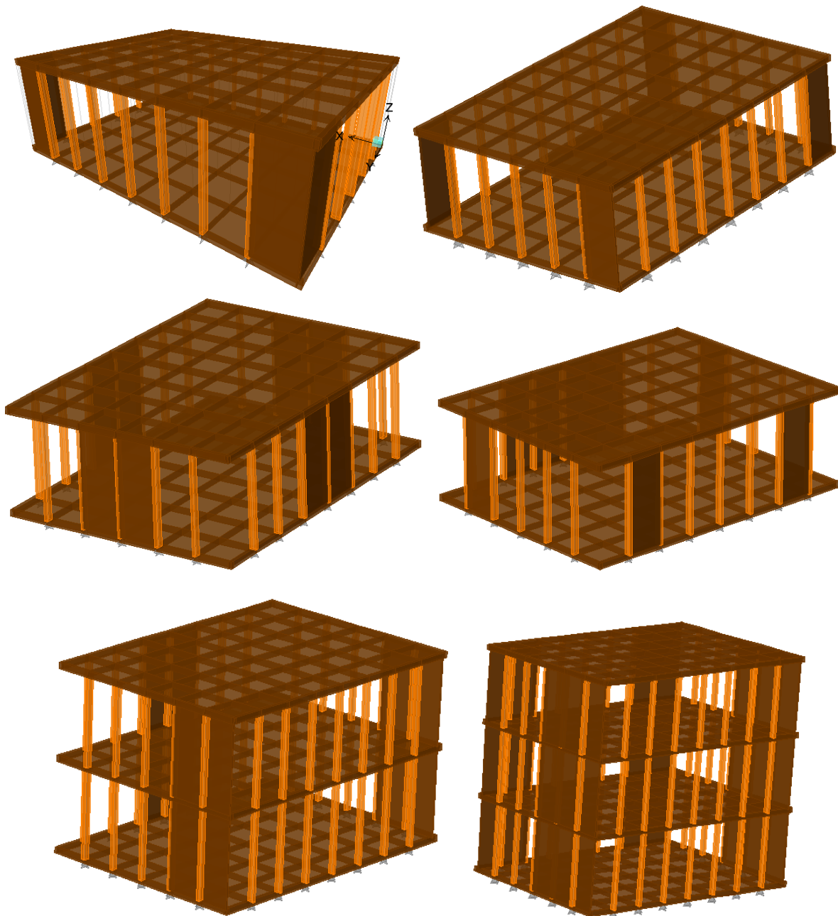
Figure 28 - Variations of GLT walls placements
