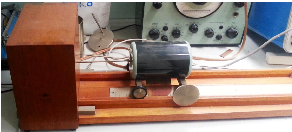
Figure 181 - Kundt's tube apparatus
