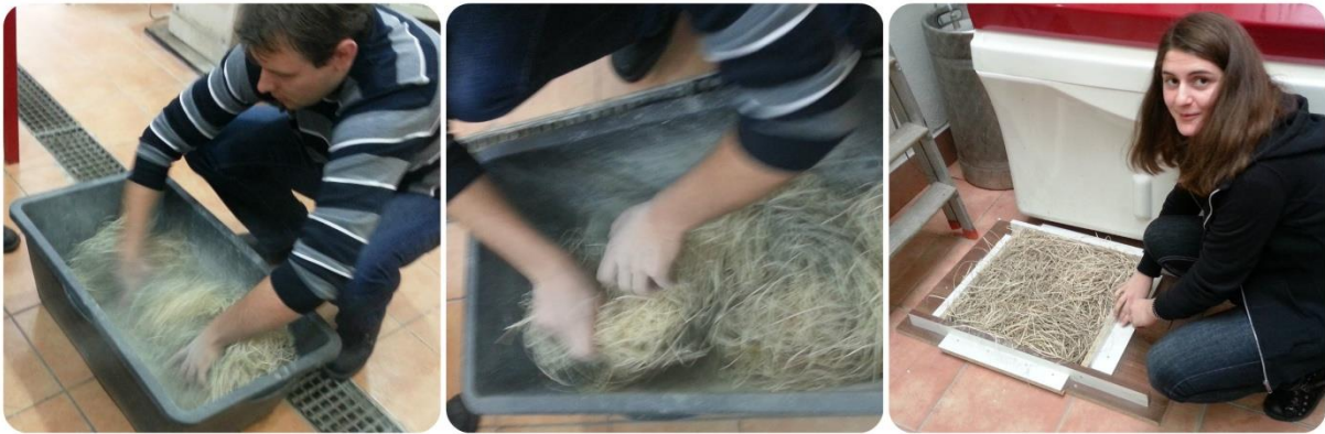
Figure 175 - Mixing the dry wood fibres with the cement
