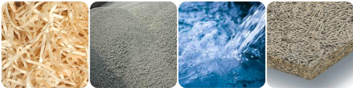
Figure 171 - Main components of Wood Wool panels: wood fibres, cement and water
