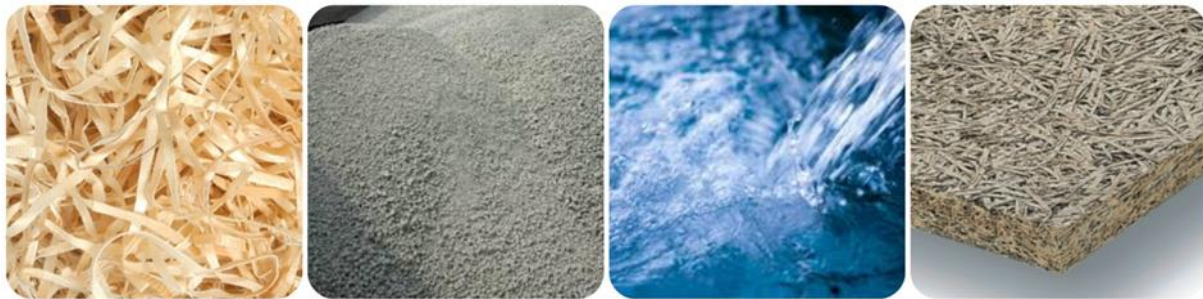
Figure 194 - Main components of Wood Wool panels: wood fibers, cement and water
