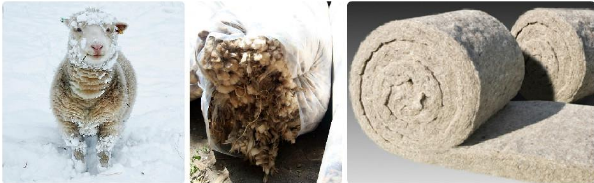
Figure 30 - Sheep wool insulation
