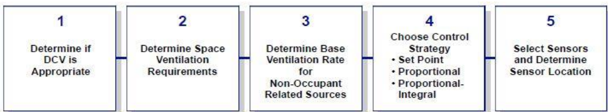
Figure 147 - Ventilation control scheme
