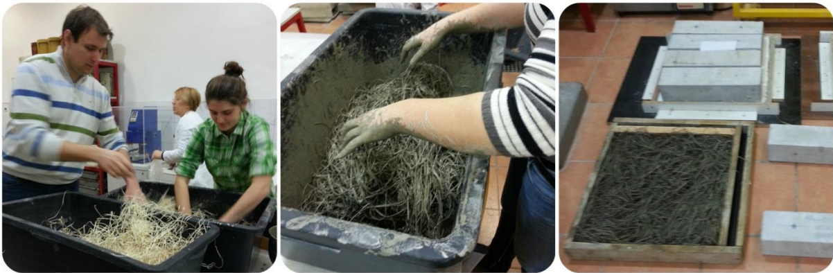
Figure 176 - Mixing the dry wood fibres with cement slurry
