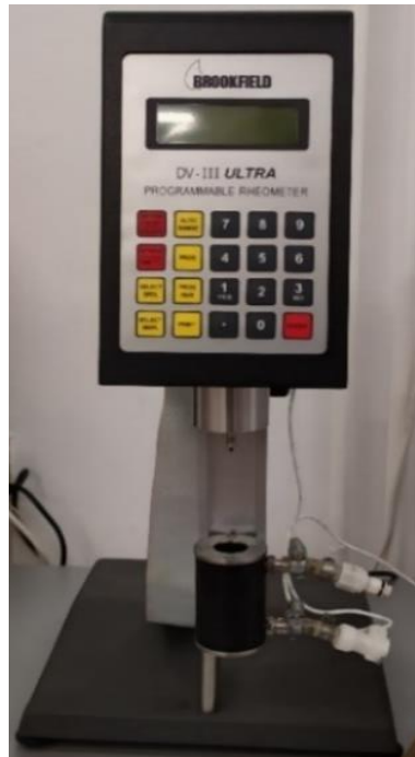
Slika 6. Viskozimetar Brookfield DV-III Ultra Programmable Rheometer.
