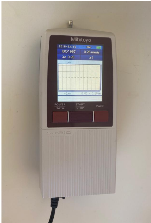
Slika 8. Uređaj Surfrest SJ-210 Surface Roughness Tester (Mitutoyo Corporation, Sakado, Japan)
