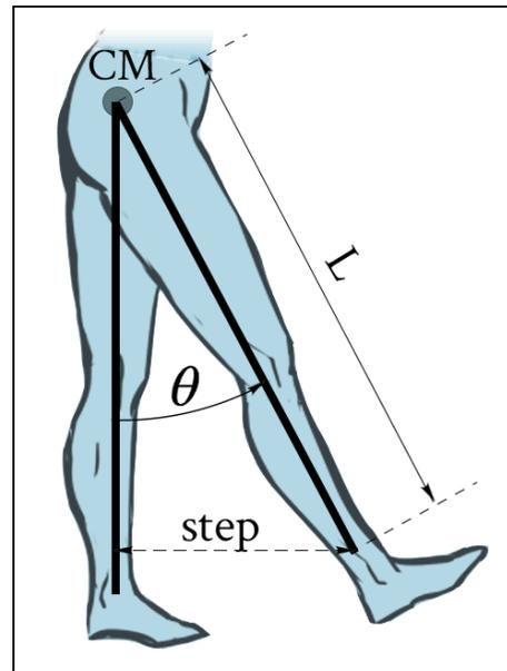
**Figure 3** A sketch of our pendulum model. The legs have length  $L$  and are separated by an angle  $\theta$  before each step.
